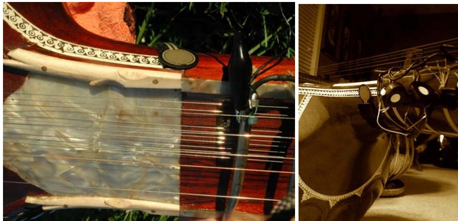
Figure 44 - FSR sensor used to measure thumb pressure on ESitar 1.0 (left) and ESitar 2.0 (right).
