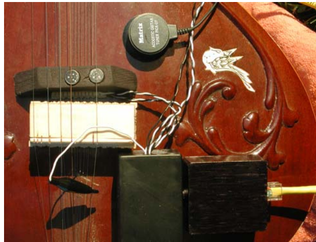
Figure 45 - Gesture capturing sensors at base of ESitar 1.0.
