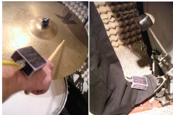
Figure 54 – Wearable sensors used for a drum set performance.
