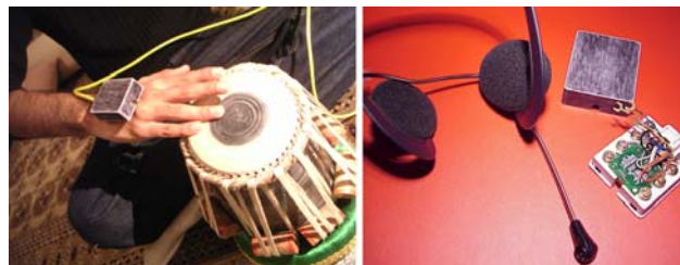
Figure 55 - Wearable sensor used for a Tabla performance (left). Set up for using on head of performer (right).
