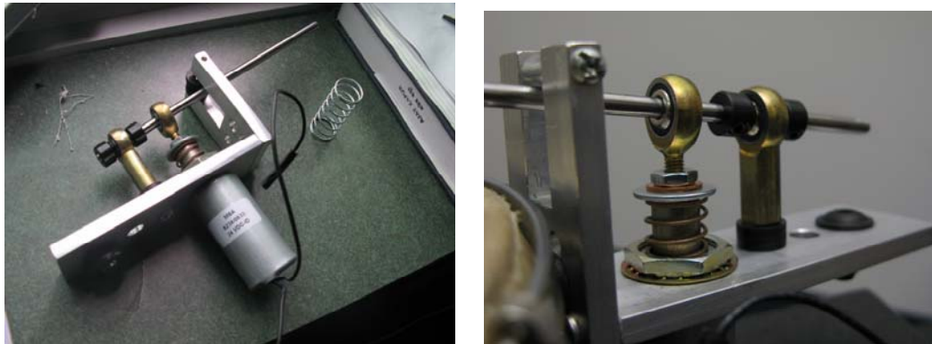
Figure 61 - Trimpin Hammer modified to fit the MahaDeviBot schematic.
