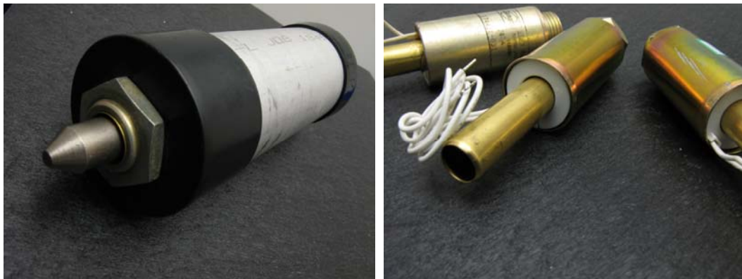
Figure 63 - Trimpin BellHop outside shell tubing (left) and inside extended tubing (right).
