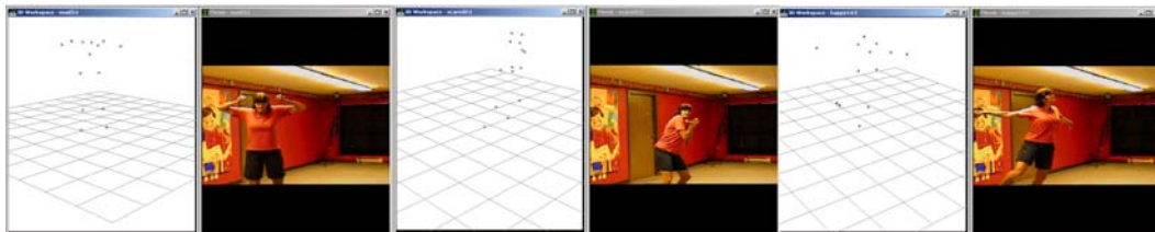
Figure 85 - Screenshot of the data capturing process. The dots on the screen correspond to the markers taped onto the human body.
