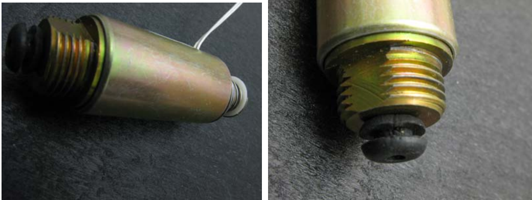
Figure 59 - Kapur Finger using a grommet and padding.
