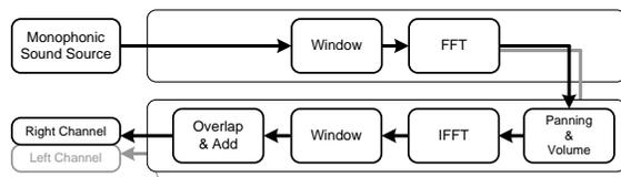
**Fig. 4:** Block-diagram of the FFT-based synthesis and panning module.
