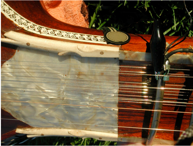
Figure 7. Picture of FSR sensor used to measure thumb pressure
