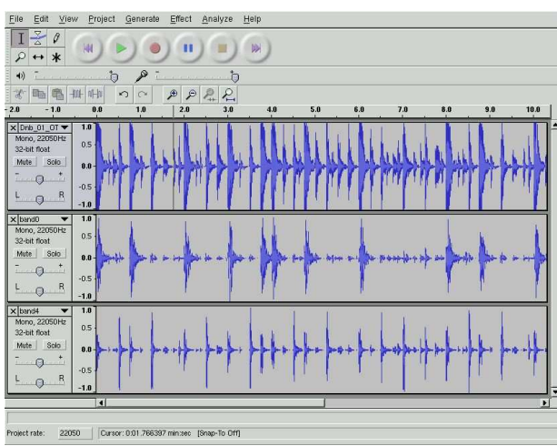
Figure 6. Original signal followed by low and high wavelet bands showing the separation of bass drum sounds from high-hat sounds
