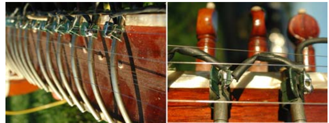
Figure 10. The network of resistors on the frets of the ESitar.
