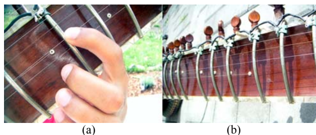
Figure 2: (a) Traditional fingers playing fret technique; (b) Network of resistors on the frets of the ESitar .
