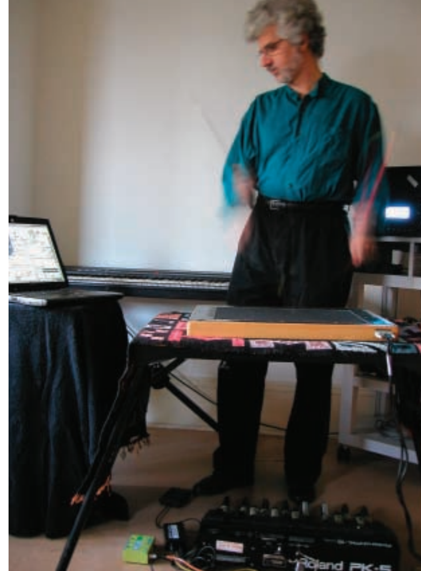
Facing page: Peter Driessen PEng in his University of Victoria laboratory testing the response characteristics of the radio drum, an electronic musical instrument that detects the performer's movements to control and trigger sound (photo: UVic). Left: Andrew Schloss performs on the radio drum in his home studio using Max/MSP, a language designed for real-time music programming (photo: Irene Mitri).
