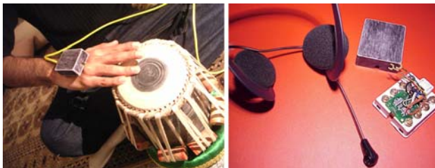
Figure 3. Wearable sensor used for a Tabla performance (left). Set up for using on head of performer (right).
