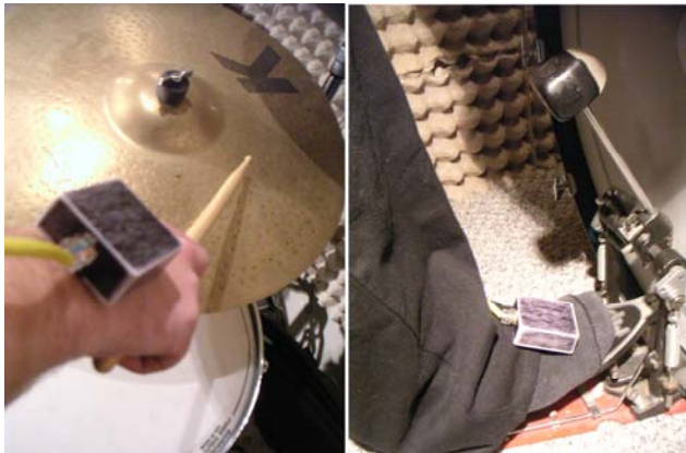
Figure 2. Wearable sensors used for a drumset performance
