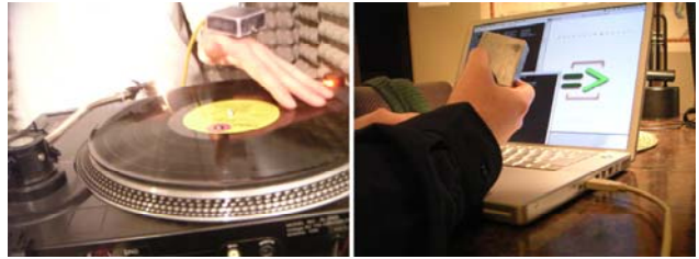
Figure 4. Wearable sensor used to capture scratching gesture of turntablist (left). Wearable sensor used in conjunction with live Computer Music Performance using ChuckK (right).
