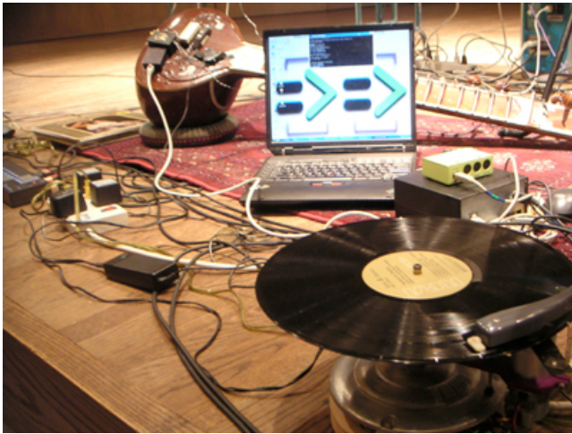
Figure 6. ESitar controller using ChuckK to communicate with Trimpin's eight robotic turntables.
